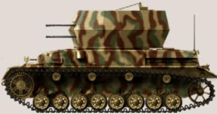
The Wirbelwind was a development of the Panzer IV designed to provide a vehicle offering AA fire support, armed with the standard 20mm AA gun quadruple mounting.
