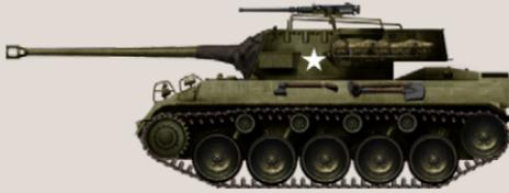
In contrast to the M10 and M36 tank destroyers, which used the heavy chassis of the M4 Sherman, the M18 Hellcat was designed from the start to be a fast tank destroyer. As a result, it was smaller, lighter and significantly faster, but carried the same gun as the Sherman 76 mm models.
