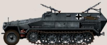
The SdKfz 251 Mittlerer MG was a German armored half-track which could bring a squad of 10 soldiers into battle alongside the tanks. It provided reasonable armor protection against small
