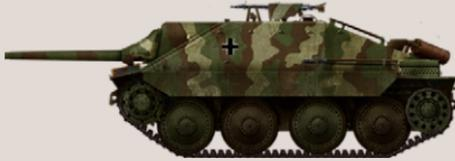
The Hetzer was a development of the Panzer 38t, designed to provide a light but powerful anti-tank weapon armed with the 75mm L48 gun. Many
