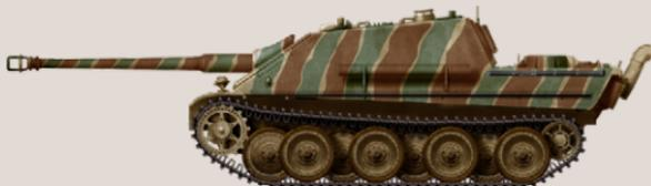
The Jagdpanther was a development of the Panzer V designed to provide a low and powerful anti-tank weapon armed with the famous 88mm L71 gun. It was a monster tank, capable of obliterating anything the allies could throw at it.
